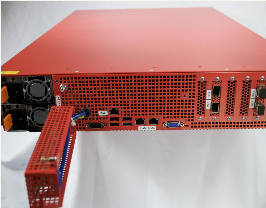
40Gb/s Storage Appliance with 248TB storage (2RU form factor)
